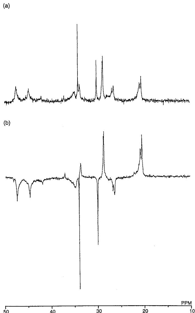
Figure 9. ^{13}\text{C} NMR spectrum (a) and DEPT spectrum (b) of propene/1,7-octadiene copolymer obtained with 2 (run 27).
